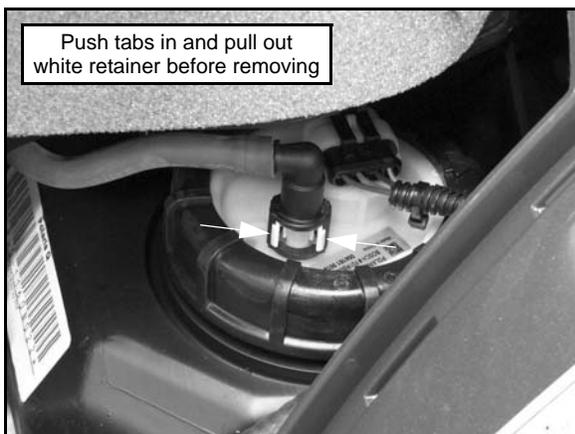
4. Lift up on the fuel line and remove it from the pump outlet.
