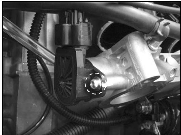
6. Rotate the TPS until your voltmeter reads within the specification (see Figure 3-20).
