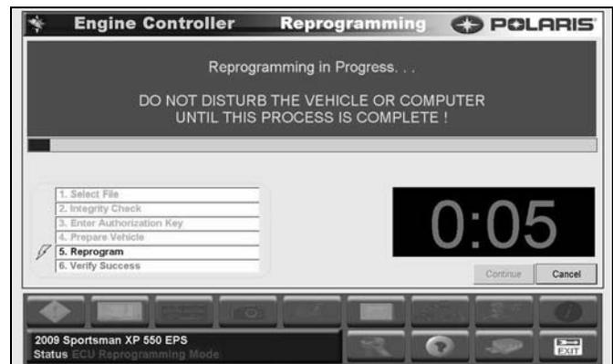
15. Once the ECU reprogramming procedure is complete, click the ‘Finish’ button on the screen. Verify the reflash was a success by starting the vehicle.
