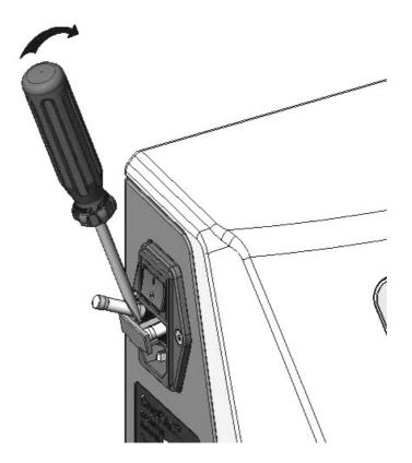
Fuses should only be replaced with the same type and rating.
