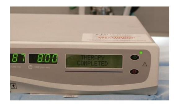
15. Controller automatically terminates heating at end of therapy cycle. Total treatment time will be displayed on controller (preheat time + therapy time).
