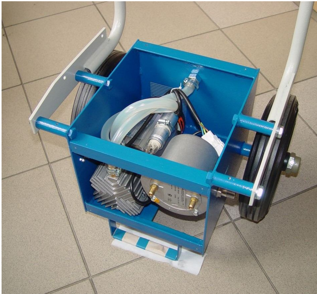
Figure 3.2 – Removing the front and upper panel of the unit
