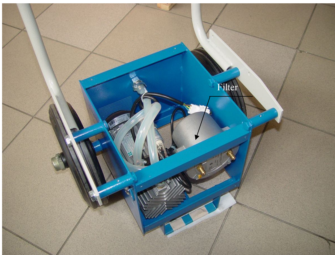
Figure 3.4 – Replacement of the filter element
