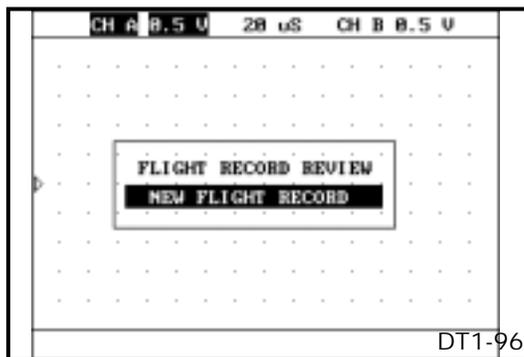
NEW FLIGHT RECORD - Pressing the ENTER key prompts you to "press any key to start recording". Press any key to stop the recording.
