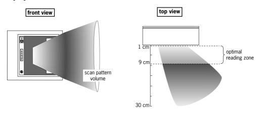
Scanning a bar code label in fly by mode is very simple: pass the product's bar code label along the scanner as illustrated in the figure below.
