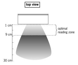
Scanning a bar code label in presentation mode is also very simple: present the product's bar code label to the scanner as illustrated in the figure below.
