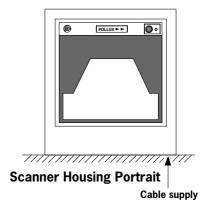
Independent from the installation you can direct the scan pattern in a way that suits your application most, thanks to the four directional optical assembly. For turning the optical assembly please refer to the Pollux Service Manual (authorized personnel only).
