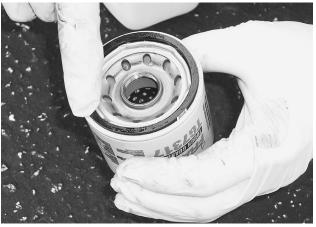
☐ Read the instructions on the filter. Install the oil filter by rotating it clockwise by hand. Once the gasket contacts the engine, tighten it according to the instructions - usually 1/2 to 1 full turn. A filter wrench may be necessary. Do not over tighten.
