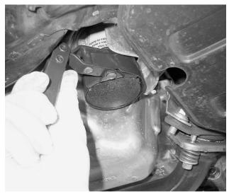
☐ Finish removing the oil filter by hand. Set the oil filter in the oil drain pan so the oil can drain out of it.
