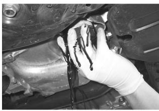
☐ Make certain the old oil filter gasket comes off with the old filter. If it is stuck on the oil filter mounting base, remove and discard it.
