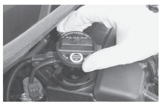
☐ Using a funnel, pour the correct amount and type of oil into the filler opening. (Make sure the API and SAE ratings match what is listed in your owner's manual.)
