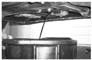
☐ While the oil is draining, use an oil filter wrench to loosen the oil filter.
