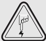
DO NOT TOUCH the print head or the electronic components on the print head carriage. Discharges of electrostatic charge from the human body or other surfaces can damage the print head or other electronic components used in this device.
