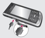
**NOTE:** KF750 should be inserted the charger to the direction which is not shown the Inserting mark.
