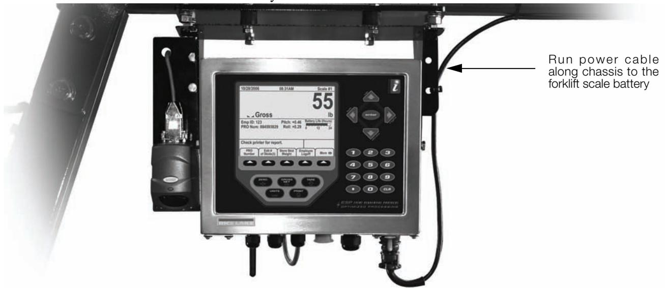
Figure 3-5. Run Power Cable to the Forklift Battery
