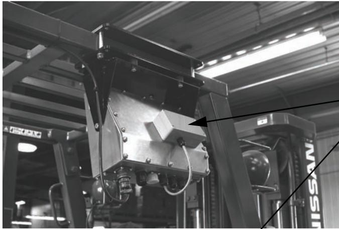
Wireless communication between the 920i indicator and the two-channel iQube which is located on the forklift and is powered by a lithium-ion battery housed in a battery box.
