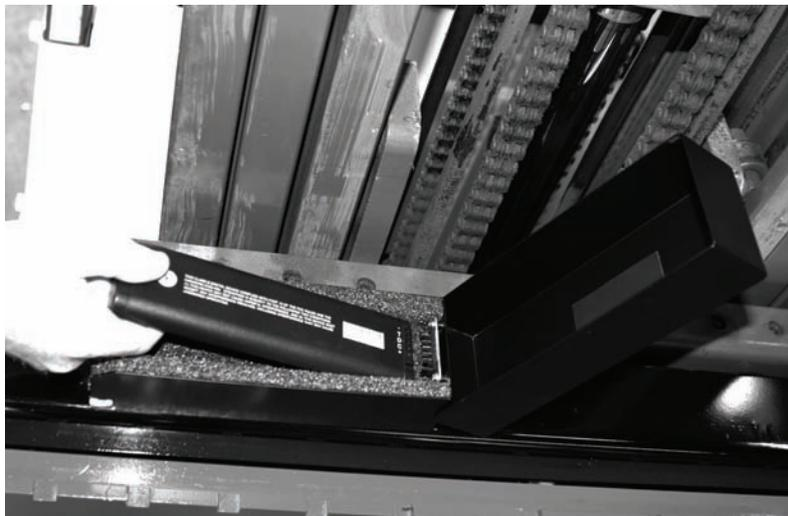
*Figure 3-12. Pulling the Lithium-Ion Battery Out*
