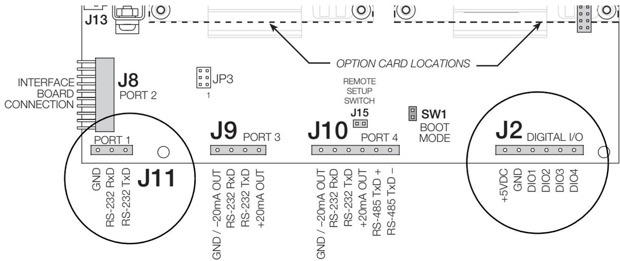
Figure 9-3. 920i CPU Board Pin Locations for Connecting the Scanner
