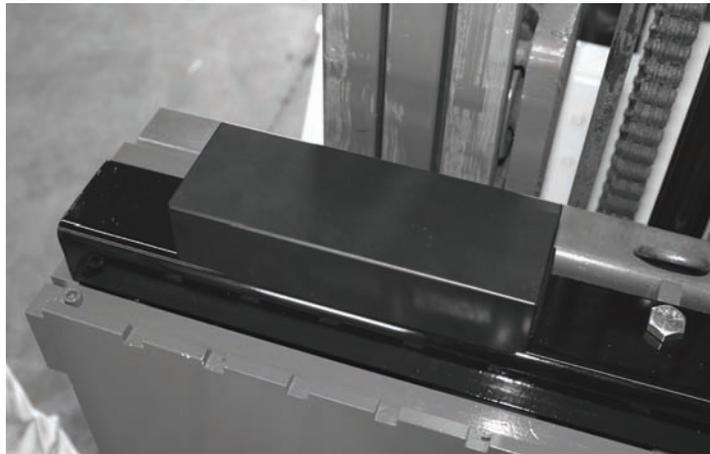
Figure 3-9. Lithium-Ion Battery Location
