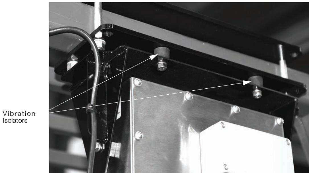
*Figure 3-2. Vibration Isolator Control Location*
