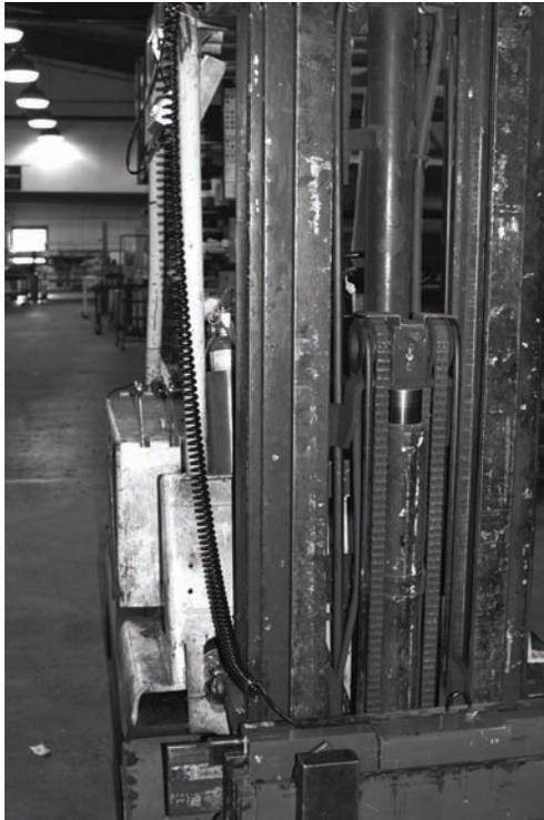
*Figure 3-8. Signal Cable Located Between the Scale and the Indicator*
