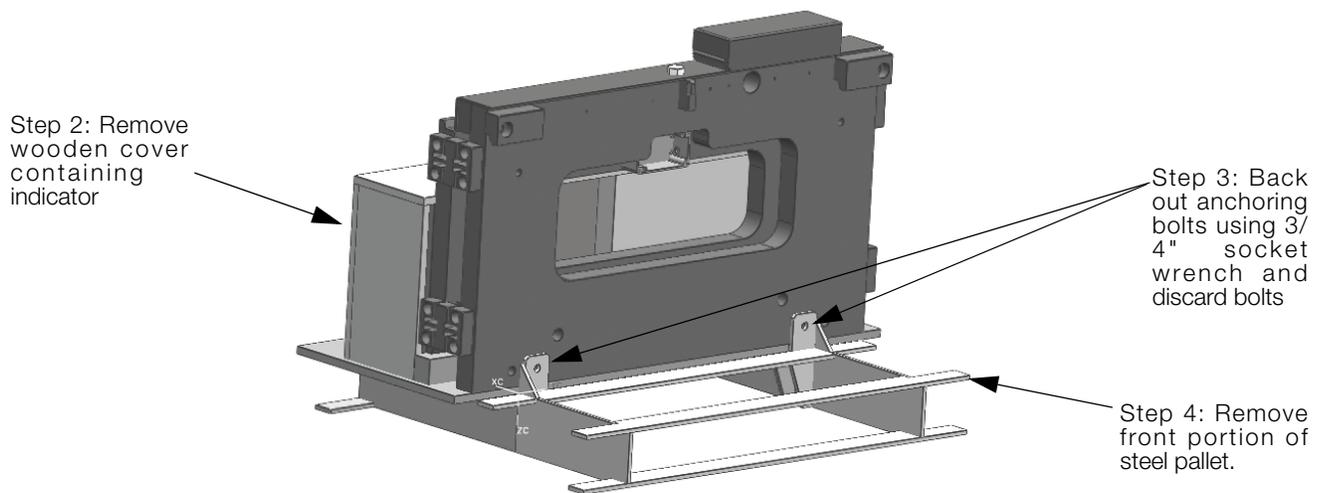
Figure 2-3. Bolt Location on Pallet
