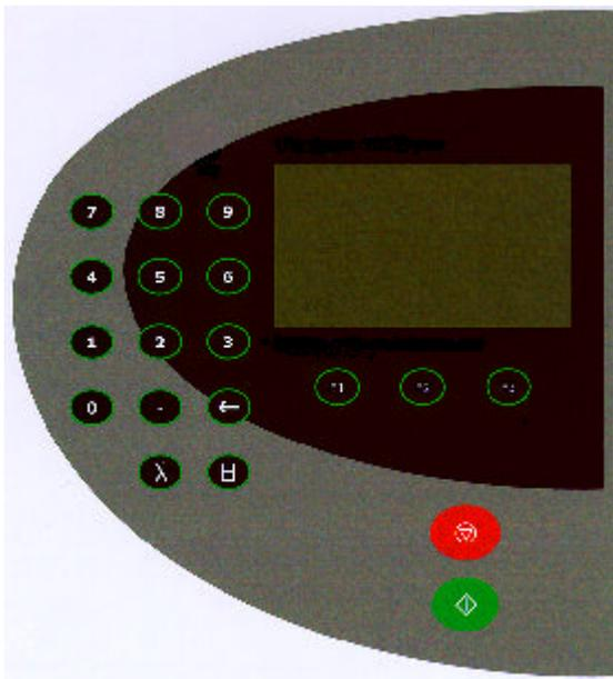
The instrument is easy to use, with function select / entry soft keys on the keypad (F1, F2 and F3) being situated directly below the corresponding option on the display; these keys are used in conjunction with on-screen prompts.
