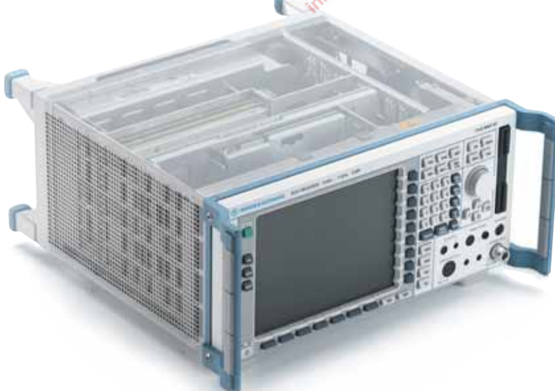
Interior view: modular design of test receiver
