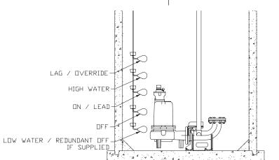
Install the ON / LEAD floats a minimum of 4 inches above the OFF float. If additional volume is to be pumped on each cycle or if the pump running time for each cycle needs to be increased, then increase the distance from the ON / LEAD float to the OFF float as needed.
