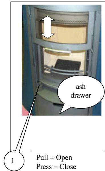
The **secondary draft control** lever regulates the amount of air that is needed to reburn exhaust gases that are produced in the fireplace during the wood burning process. A portion of this secondary air circulates from the top to the door and helps to keep the glass window clean.
