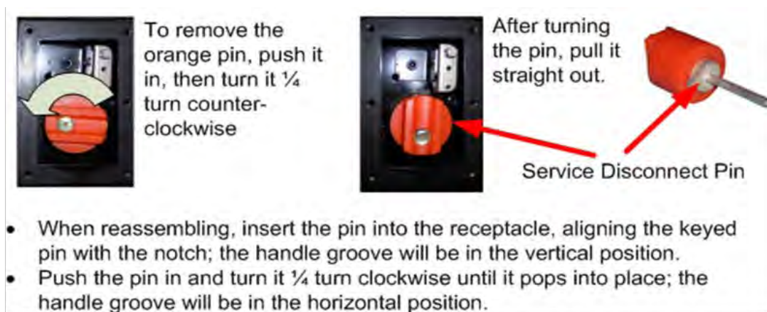
Figure 61: Removing high voltage service disconnect pin
