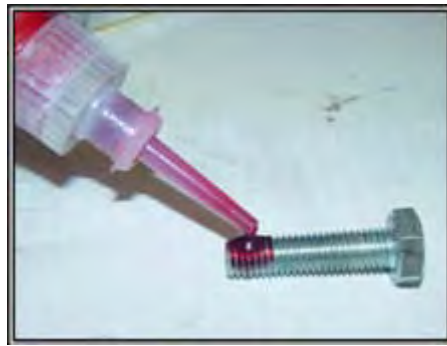
Applying Loctite® product on screws
