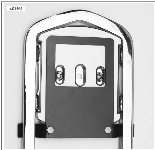
Figure 4. Bracket for 2.55 Inch (64.8mm) Pad Hole Spacing (Lamp Assembly Installed - View from Front of Sissy Bar)
