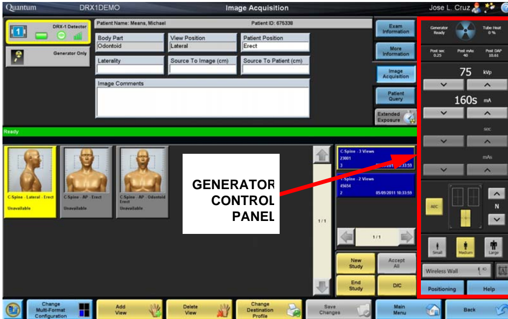
Figure 3-5. Quantum Q-Rad Generator Control Panel Integrated with CR/DR System's Workstation Computer
