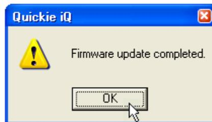
**After a firmware update it is now necessary to restore the drive profile parameters that you saved, refer to section 3.5.5 Loading File Stored Data**
