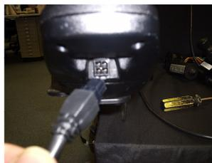
The CAN Harness may be plugged into any convenient bus connector on the wheelchair; this would normally be at the front of the hand control module (joystick).
