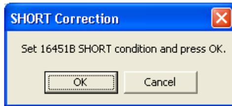
After setting the 16451B SHORT condition as shown below, press “OK” to perform the SHORT correction for electrode adjustment. A message “Done” is shown in the blue area below the “Cable length correction” button when this step is completed.
