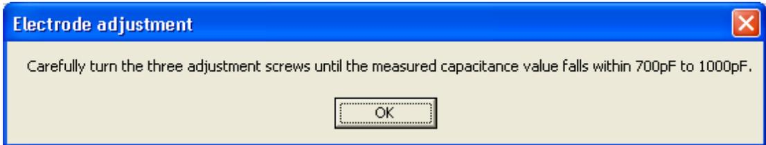
Adjust the Unguarded electrode by turning the three adjustment screws until the measured Cp value falls within the limit. The details about the adjustment are described in the paragraph “Accurate Adjustment to Make Electrodes Parallel” in Chapter 3 of the 16451B Operation and Service Manual.
