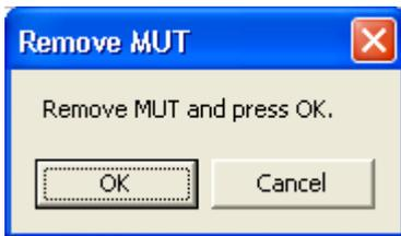
Remove the MUT and click “OK” button. The capacitance and dissipation factor measurements without the MUT inserted are performed. After the measurement, the calculated dielectric constants are automatically displayed in the sheet.
