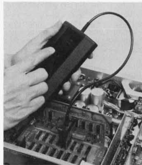
Figure 8. 10529A Logic Comparator. An IC is checked during in-circuit operation.
