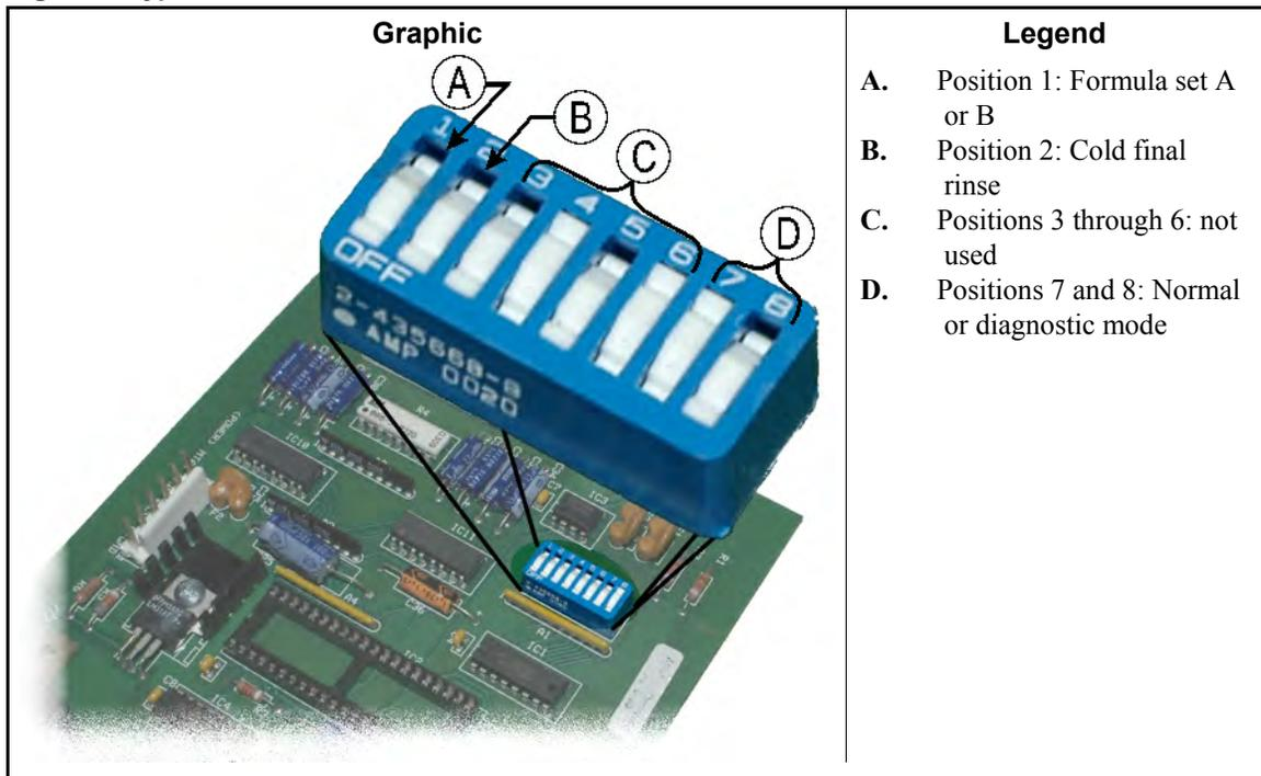
Figure 7: Typical DIP switch on 08BT168BT
