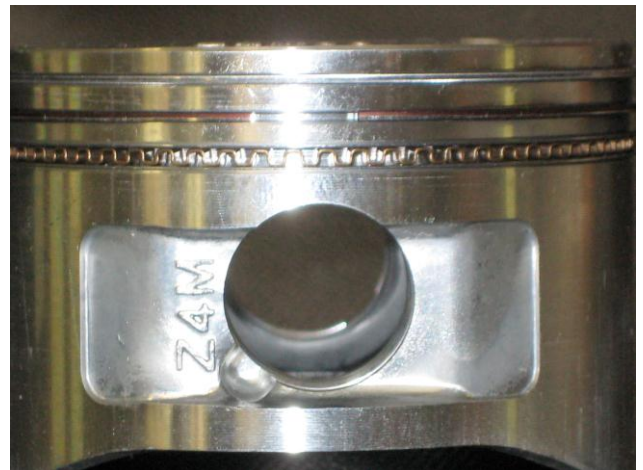
SIDE VIEW GX160 UT1 PISTON (13101-Z4M-000)
