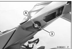
Prepare the rear frame [B] surface around the front grab rail mounting bolt ends [A] using a suitable cleaning fluid to remove any oil or dirt on the frame near the mounting bolt ends, and dry with a clean cloth.
