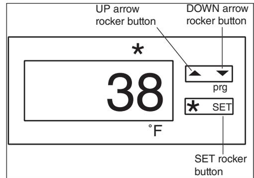
The controller is pre-programmed with a 34 F set point which provides a compressor cut-in at 38 F and cut-out at 34 F. This may not meet your specific application needs. For example, many pharmaceutical manufacturers recommend that their refrigerated medications be stored between 36 F and 46 F. Instructions for changing the set point are found below.
