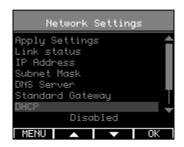
4. Use the UP button to select IP Address and press OK.
