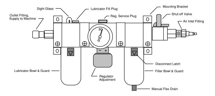
After connecting your air supply, turn the shut-off valve to the ON position. Proper air pressure (80-90 PSI) can be obtained using the regulator adjustment knob.
