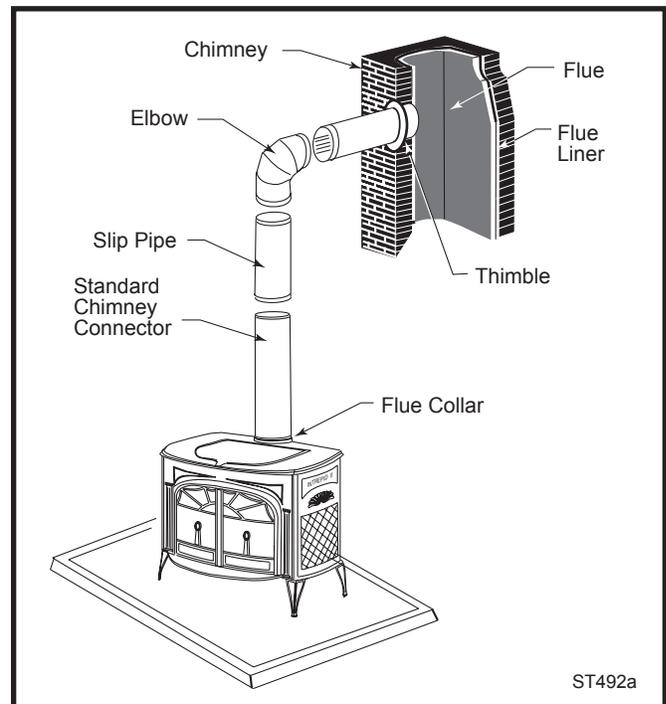
**Fig. 4** Chimney connection in a freestanding installation.
