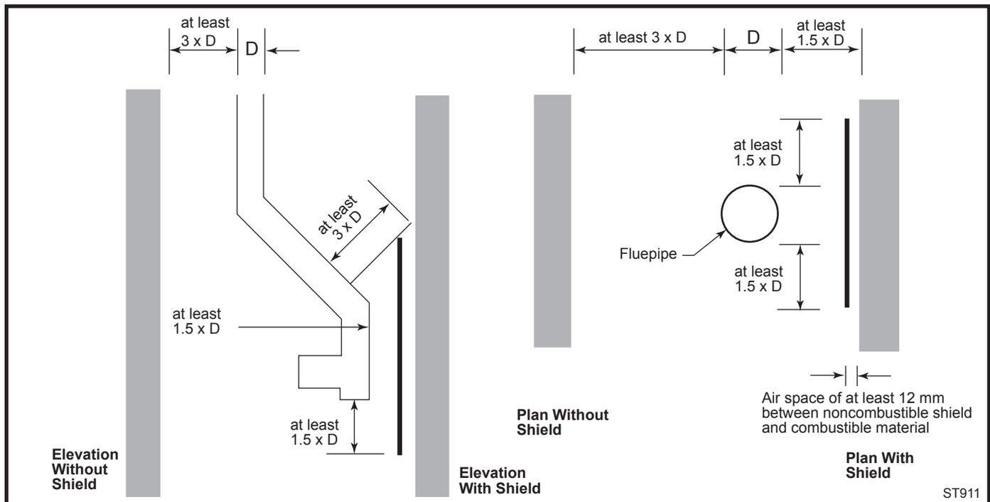
Fig. 12 Connecting fluepipe clearances.
