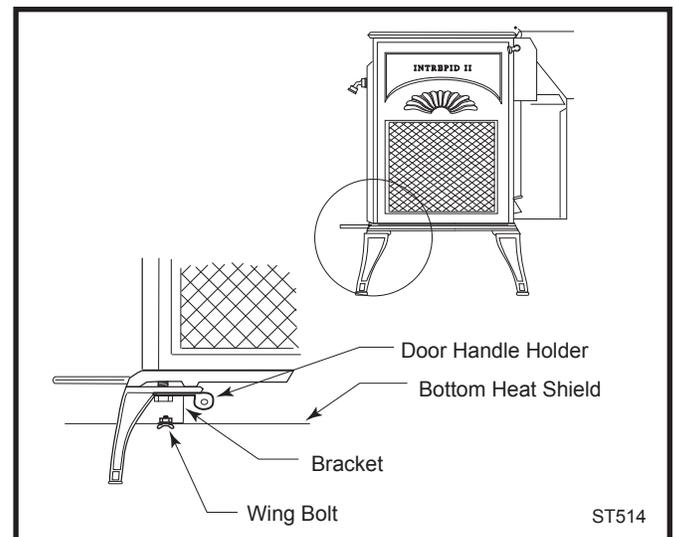
Fig. 15 Handle holder and heat shield positions.
