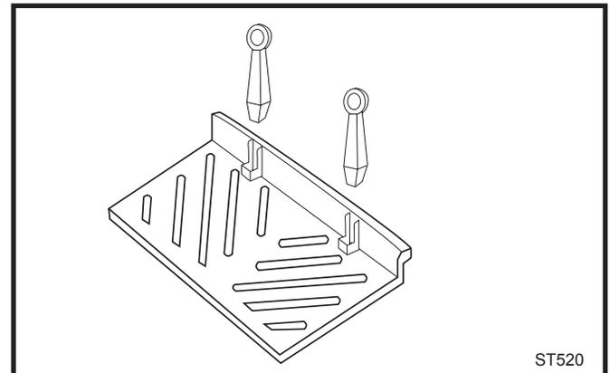
**Fig. 21** Remove the andirons for front loading.
