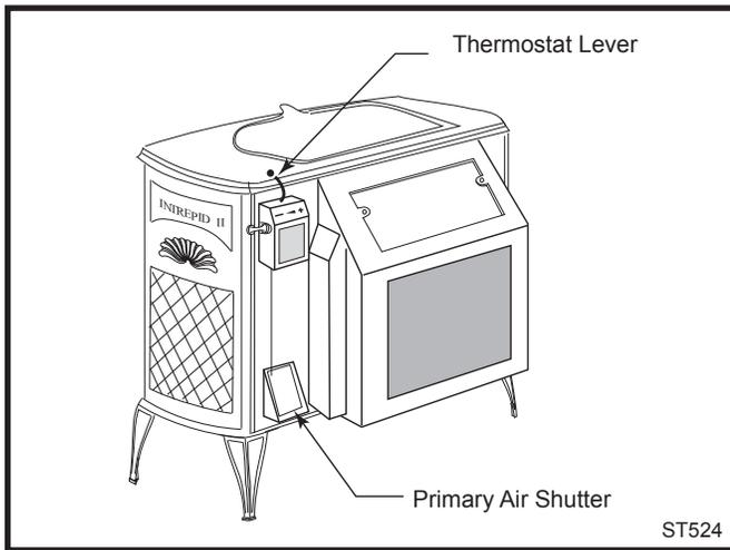
**Fig. 29** The primary air shutter must move freely.
