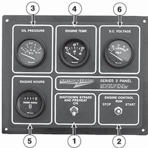
Figure 4-A: Series 3 Generator Control Panel
