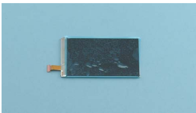
21. Protect the DISPLAY with protective film.
