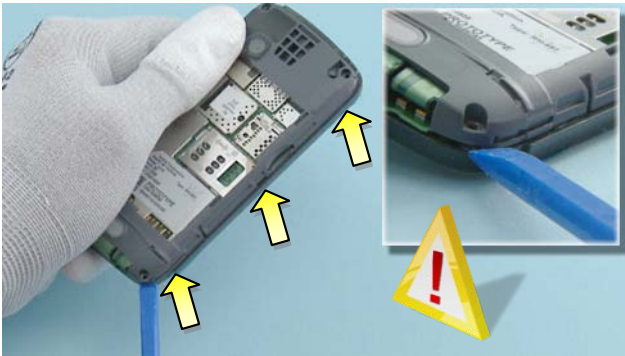
13. Detach also the clips on the other side, as shown.
