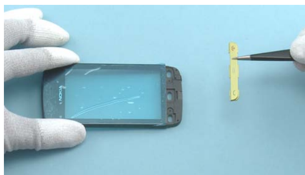
24. Remove the KEYMAT with the tweezers.
