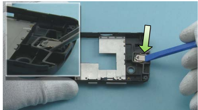
6. Place the EARPIECE with the tweezers and push it down with the SS-93 to activate the adhesive.
