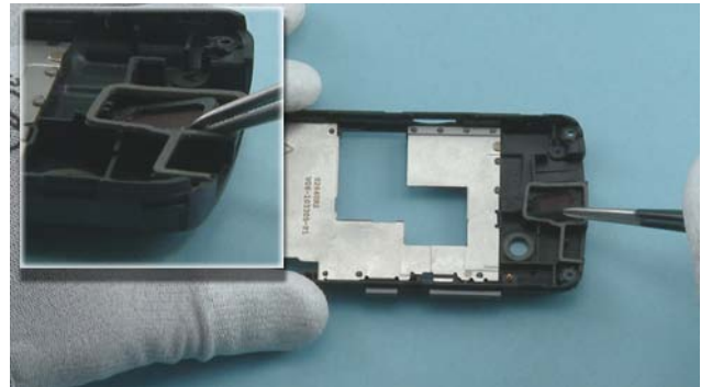
4. Place the EARPIECE ADHESIVE to its place with the tweezers.
