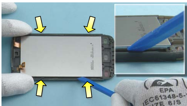
19. Use the SS-93 to carefully detach the DISPLAY from all sides.
