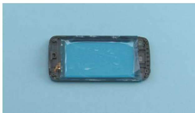
22. Protect also the TOUCH PANEL from the inside with protective film.
