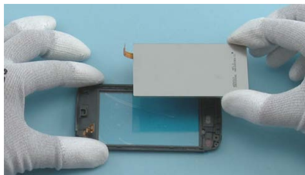
20. Lift the DISPLAY away from the FRONT COVER ASSEMBLY.
