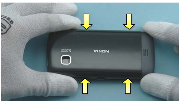
23. Insert the BATTERY and place the BATTERY COVER to its place. Press it gently to lock up the clips.
