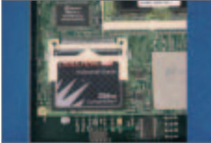
Figure 23. The compact flash can now be removed, reprogrammed & replaced
