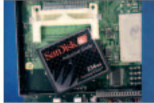
Figure 23. The compact flash can now be removed, reprogrammed & replaced
