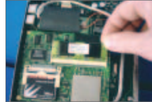
Figure 24. 24 RAM can also be accessed if necessary (Observe E.S.D. precautions)
