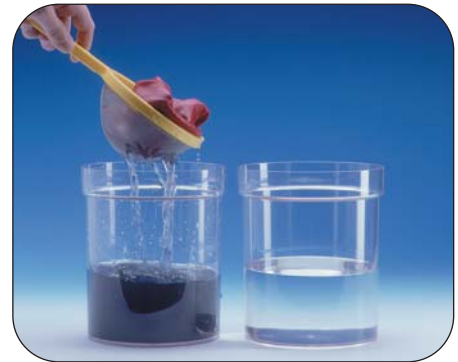
You can see the effect of total top transfer vs. other methods by using buckets of water to simulate different compartments. A Milnor loading scoop lifts the goods, drains them, and deposits them into cleaner water.
