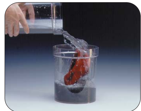
Other tunnels send dirty water into the next compartment, along with the goods. There's no dilution as the whole compartment moves forward.
