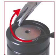
14. Remove the retaining C-ring by using the appropriate removal tool and pincer.
