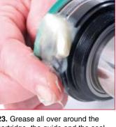
23. Grease all over around the cartridge, the guide and the seal with the special grease supplied with the kit.
