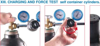
36. Adjust the required maximum pressure trought the regulation valve. The gauge on the right will pressure to charge the cylinder. 39RP pressure regulation valve.
