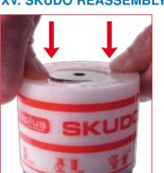
46. Manually reassembly the protective cap SKUDO on the proper groove on the top of the rod. It would be required a light pressure to correctly position it. When the protective cup SKUDO enter correctly into the groove you will hear a loud like "CLICK".
