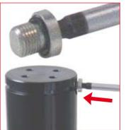
43. thread the protective screw into the charging hole by using the appropriate tool. 58CE05 for 1/8G charging port. **58CE03** for M6 charging port.
