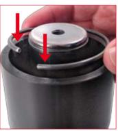
26. Position the retaining C-ring into the conical centring guide tube.
