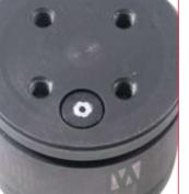
**34.** Once re-positioned the OSPAS device set the aluminum seal on the hexagonal hole and smash it. It is severely forbidden to press the piston-rod into the body when the safety device OSPAS is positioned. High risk to damage and compromise the functional of the safety
