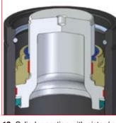
**12.** Cylinder section with piston/rod and cartridge completely pressed into the body.
