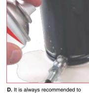
check leaks on all connection to and from the cylinder by using the special gas detector. 39RFG Special Springs gas detector.
