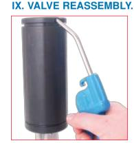
19. Carefully clean the lodging hole of the valve with an airgun and then position the new one way valve supplied along with the maintenance kit. Be care on the right position of it.
