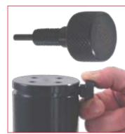
3. Thread DDS bleed device on the charging port then exhaust completely the pressure. Point away from the operator for maximum safety. DDS-1/8G for the 1/8 G port.
