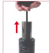
15. Manually extract together piston/rod/cartridge from the cylinder body. It would be required some strain for certain models.
