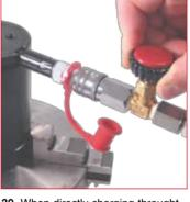
**39.** When directly charging throught the adapter and desired pressure is reached shut off the hose and bottle valves and disconnect the the quick
