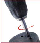
**6.** To remove the safety device OSAPS it is necessary to remove first the aluminium seal from the hex hole of the screw. Use the special drill hit, included in the maintenance kit, and mount it on a small hand drill.
