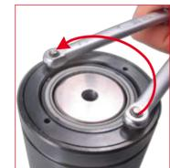
10. Remove the upper ring nut on the body by using the appropriate wrench 58CC... compass wrench.
