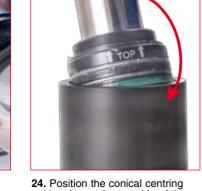
guide tube on the top side of the cylinder body, then position the piston/rod/cartridge into the tube and assure to keep all perpen-dicular to the tube itself and the 49TB... conical centring guide tube
