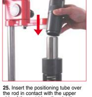
the rod in contact with the upper side of the cartridge, then by the manual press, press down into the cylinder body all the assembled parts. 49TB... conical centring guide tube. 39PM01 manual press.
