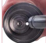
17. Carefully check and clean the cylinder body. If the body show any wear or damage do not use it again and replace it with a new one.
