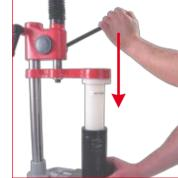
**11.** Position the anti scratch nylon removal tube on the cartridge then press down into the body for about 25 mm to set free the retaining C.
