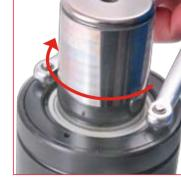
44. After the charging operation it is recommended to double check the right locking of the upper ring nut on the body by using the appropriate compass wrench.
