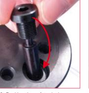
32. Position the safety device OSPAS into the proper hole located in the cylinder bottom. It is severely forbidden to press the piston-rod into the body when the safety device OSPAS is positioned. High risk to damage and compromise the functional of the safety device.
