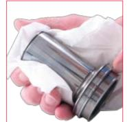
18. Carefully check and clean the piston-rod. If the piston rod shows any damage, wear or scratch do not use it again and replace it with
