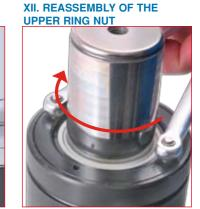
30. Position and thread the upper ring nut of the cylinder by using the appropriate compass wrench. 58CC... compass wrench.
