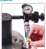
37. Select and assemble the desired charging adapter and thread it on the charging port. For an easy and safety work carefully follow the instructions supplied with the charging unit. DO NOT exceed the maximum pressure indicated for any specific model. 39DMA charging unit.
