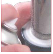
42.1. It is always recommended to check leaks on the upper side of the cylinders after the maintenance work and before re-using the cylinders by using the special gas detector.
