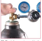
35. Check the correct assembly of the pressare regulation valve on the gas bottle, then open the main tap. The gauge on the left will indicate the bottle pressure.
