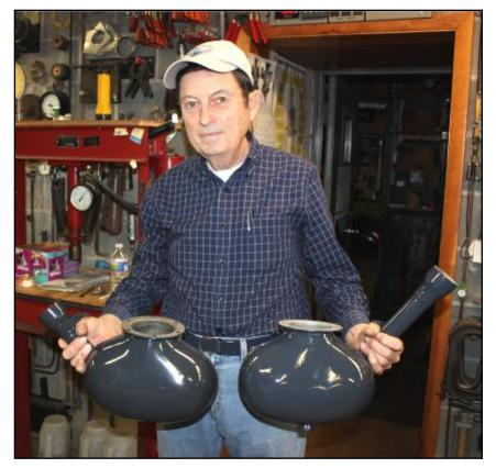
In the photo to the left Bill Pancake is holding an A50331 oil sump used on an Aeronca A-65 engine in his right hand, and an oil sump used on a Cub with a similar A65 engine in his left hand. Note the difference in the length and position of the filler neck. It should also be noted that the Aeronca sump was made from much heavier steel and weighed considerably more than the Cub sump.
