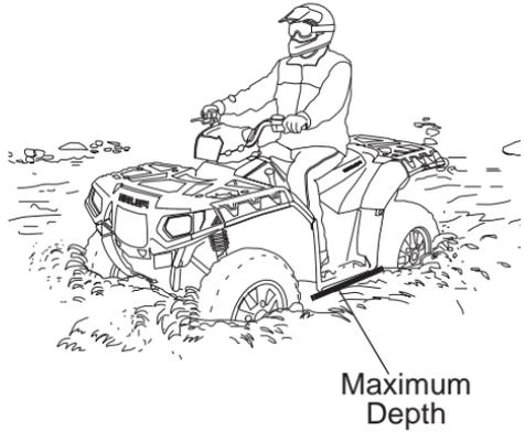
**NOTICE:** Major engine damage can result if the vehicle is not thoroughly inspected after operation in water. Perform the services outlined in the maintenance chart. See page 79. The following areas need special attention: engine oil, transmission oil, demand drive fluid, rear gearcase oil and all grease fittings.
