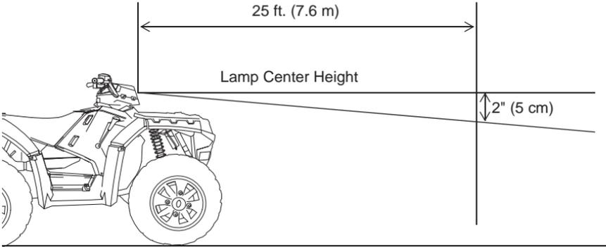
2. Measure the distance from the floor to the center of the headlight and make a mark on the wall at the same height.
