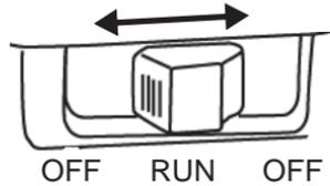
Both the main switch and the engine stop switch will shut off all electrical power to the vehicle, including lights.
