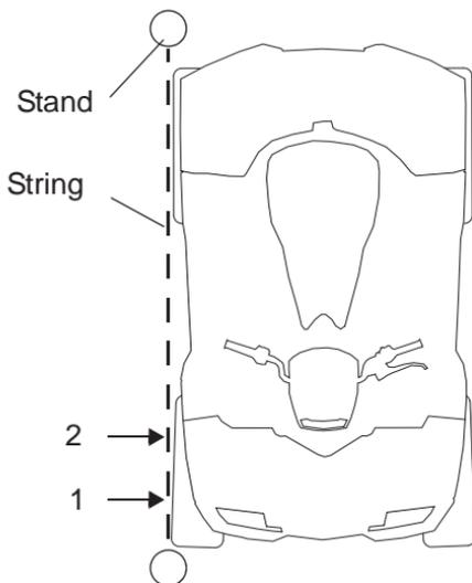
The rear measurement should be 1/8-1/4 inch (3-6 mm) more than the front measurement on each side of the vehicle to obtain the recommended 1/4-1/2 inch (6-12 mm) toe out alignment.
