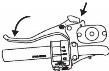
**WARNING!** Operating the ATV while the parking brake is engaged could result in an accident or fire. Always check to be sure the parking brake is disengaged before operating.
