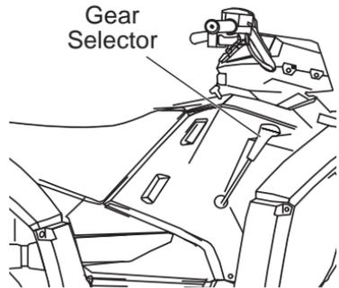
**NOTICE:** Shifting gears with the engine speed above idle or while the vehicle is moving could cause transmission damage.
