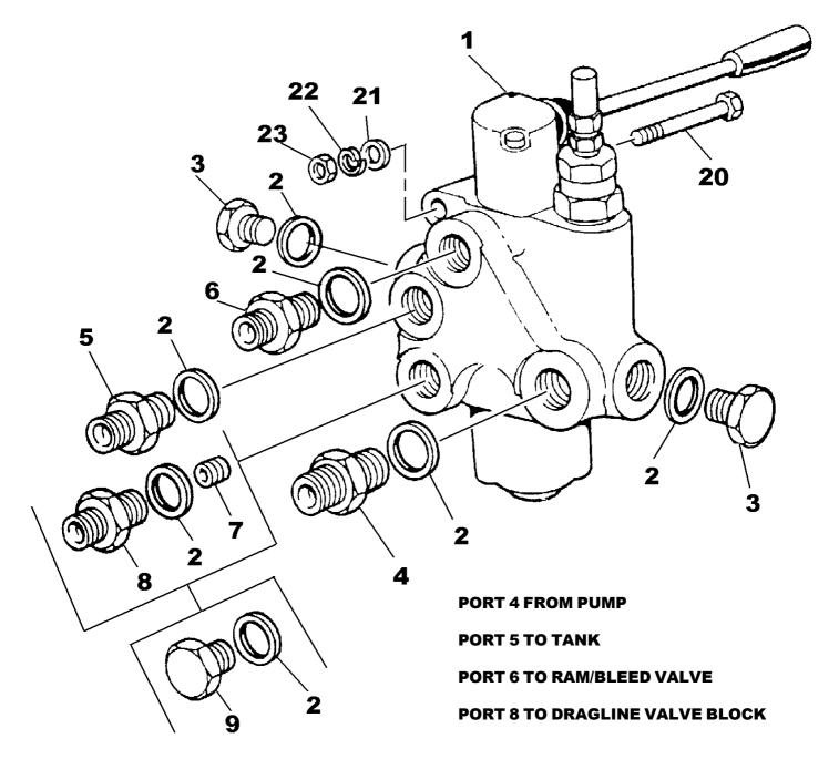
IF NO DRAGLINE IS FITTED PORT 8 IS PLUGGED WITH ITEM 9. WHEN A DRAGLINE IS FITTED, ITEM 7, THE H.P.C.O. SHOULD BE SCREWED FULLY HOME INTO THE VALVE PORT FOLLOWED BY THE ADAPTOR AND BONDED SEAL ITEMS 8 AND 2. THE THREADS ON ALL THE ADAPTORS MUST COATED WITH HYDRAULIC SEALER ON ASSEMBLY TO PREVENT OIL LEAKS
