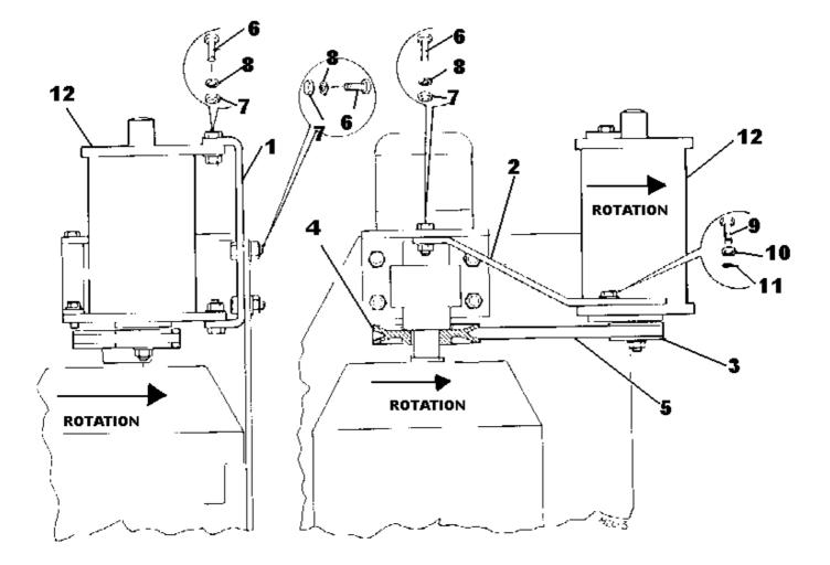
THE HYDRAULIC PUMP AND ELECTRIC MOTOR SHOULD BE CORRECTLY ALIGNED TO PREVENT PREMATURE FAILURE OF THE NYLON COUPLING SLEEVE. CHECK THAT THE TWO PULLIES ARE ALIGNED AND THE V BELT IS CORRECTLY TENSIONED
