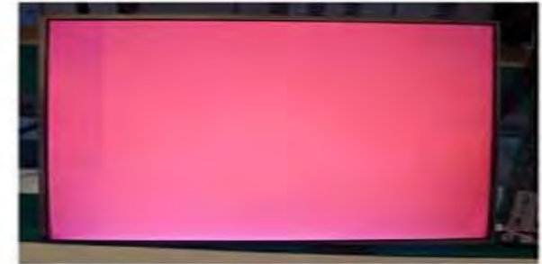
Vertical Block Source TAB IC Defect
