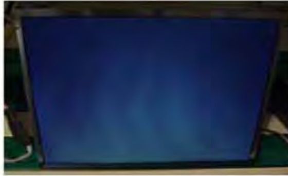
Panel Mura, Light leakage
