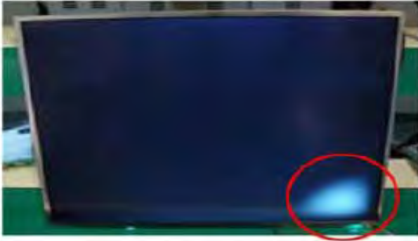
Panel Mura, Light leakage
