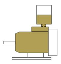
3. Fill to level indicated on the oil level label. Note this is a guide only and allowance should be made for expansion and contraction of oil during operation.
