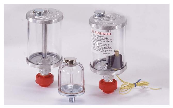
Oil reservoir assemblies easily screw in where the oil fill cap is located on all Hydra-Cell pump models D/G-03 and larger. Pumps equipped with an oil reservoir provides more volume for oil expansion and allows for quick visual monitoring of the oil level and its condition.
