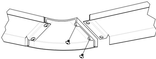
Assemble trim pieces as shown with the screws provided in the parts bag.
