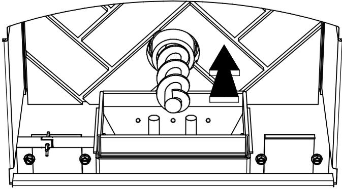
1. The Auger is packed in the hopper or ash pan and must be installed properly as illustrated below.
