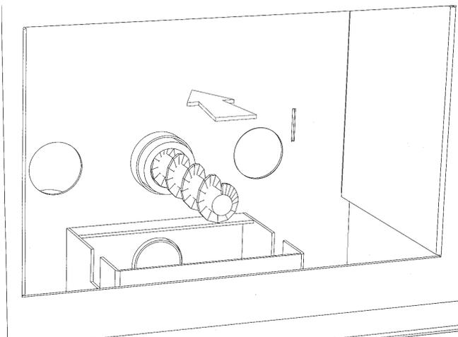
1. The Auger is packed in the hopper and must be installed properly as illustrated below.
