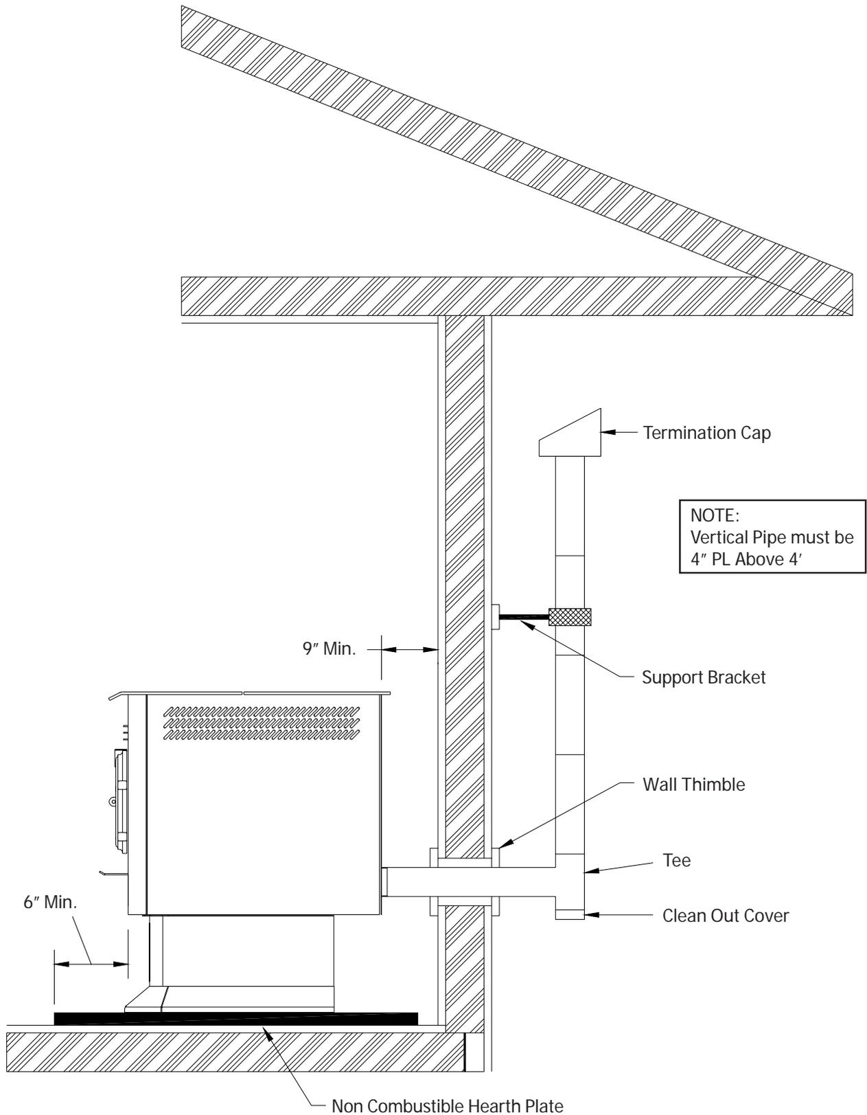
The Hearth Pad is not required under the unit if the floor is noncombustible but is required 6 inches (152mm) beyond the front of the unit and 6 inches (152mm) beyond each side of the door if the floor is a combustible floor. wood flooring, carpet, linoleum, etc.
