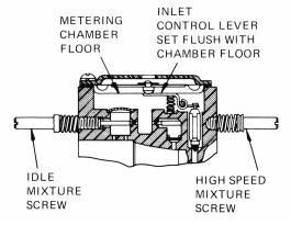
When reassembling the inlet control lever and spring, care should be taken to see that the spring rests in the well of the metering body and locates on the dimple of the inlet control lever (as illustrated above).
