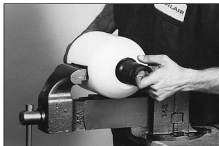
10. Slide the anti-extrusion ring off of the fluid port. Carefully fold the anti-extrusion ring until it's sufficiently folded to allow removal from the shell and remove fluid port from the shell.
