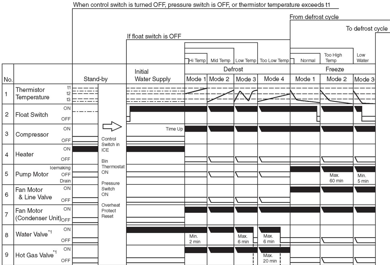
\*1 The icemaker does not complete a defrost cycle in the first 2 or 3 minutes. See "II.B.4. Controls and Adjustments."
