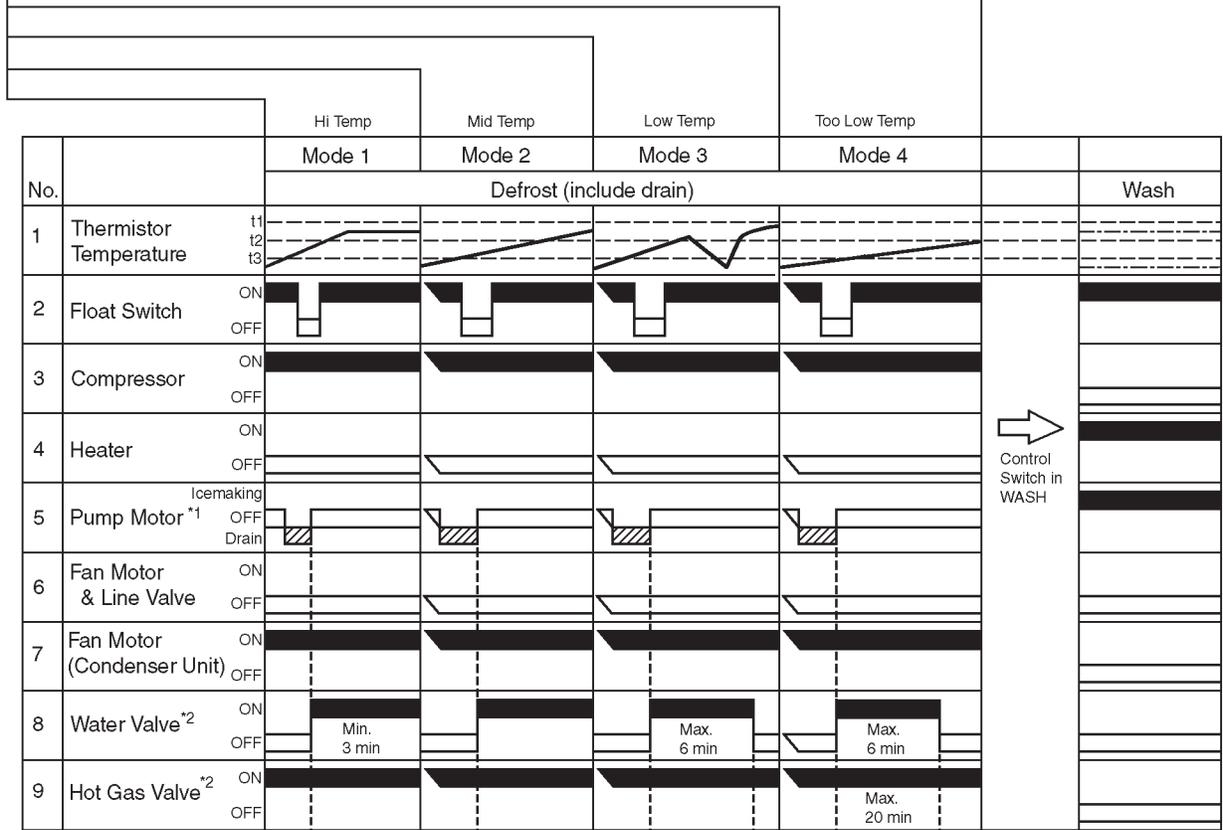
\*1 The pump motor waits for 2 seconds before starting a drain cycle. See "II.B.4. Controls and Adjustments."
