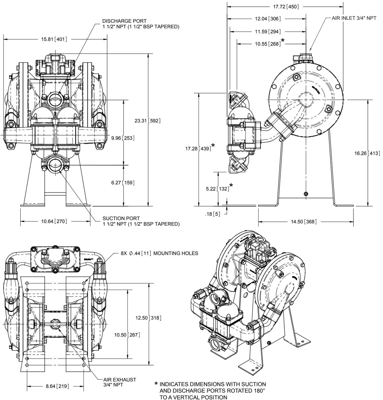
**Model HDB1½-A features 1½" NPT threaded connections.**
