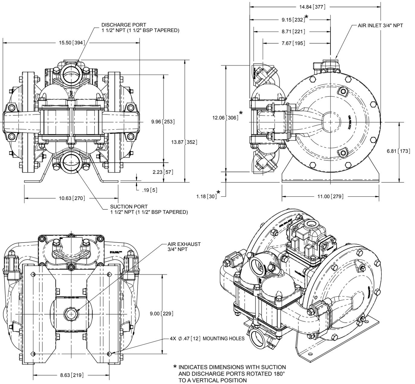
**Model HDB1½-A features 1½" NPT threaded connections.**
