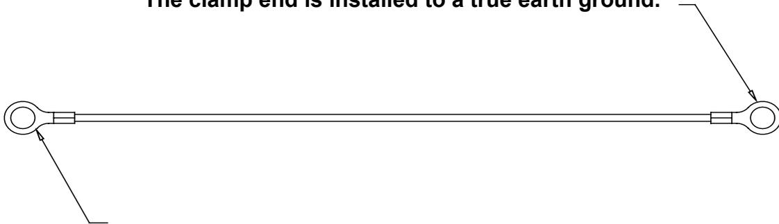
The eyelet end is fastened to the pump hardware.
