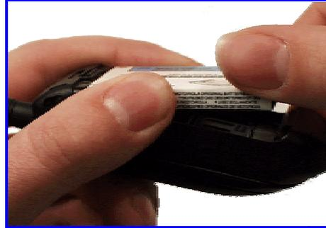
2. Remove the battery from pushing from the bottom and lifting outwards.
