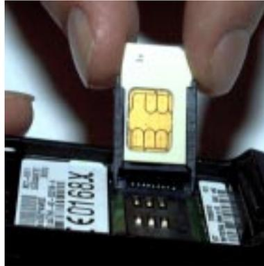
Figure 6.1 SIM Card insertion
