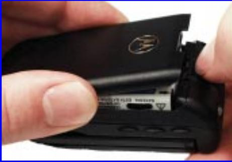
1. Remove Battery door by pressing up on latch and pulling door.
