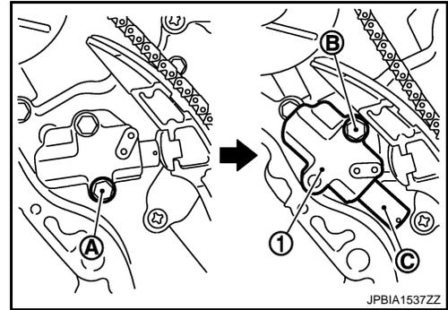
33. Remove internal chain guide (1), and slack guide (2).
