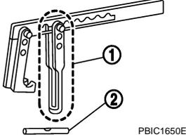
Disassembling valve mechanism<br>Part (1) is a component of KV10116200 (J26336-A), but Part (2) is not so.                                                                                                        |
