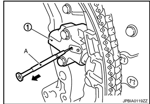
7. Check again that the matching marks on sprockets and timing chain have not slipped out of alignment.
