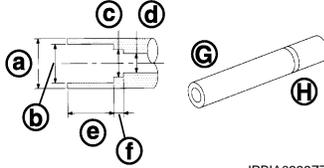
Installing valve oil seal<br><b>Use side A (G).</b><br>a: 20 (0.79) dia.      d: 8 (0.31) dia.<br>b: 13 (0.51) dia.      e: 10.7 (0.421)<br>c: 10.3 (0.406) dia.      f: 5 (0.20)<br>H: side B<br>Unit: mm (in) |
