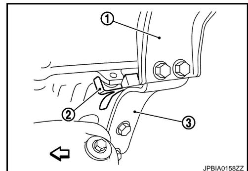
2. Remove power steering oil pump from engine side. Refer to [ST-45, "Exploded View"](#).
