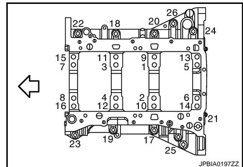
9. Remove lower cylinder block as follows:
