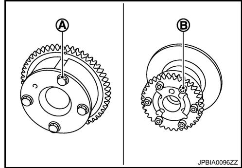
36. Remove timing chain tensioners (secondary) from cylinder head as follows, if necessary.
