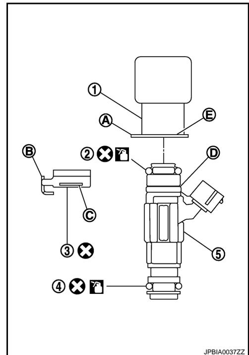
5. Install fuel tube and fuel injector assembly to intake manifold.
