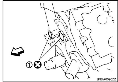
6. Remove timing chain tensioners (secondary) from cylinder head as follows, if necessary.
