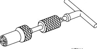
Replacing valve oil seal                                                                                                                                                                                          |
