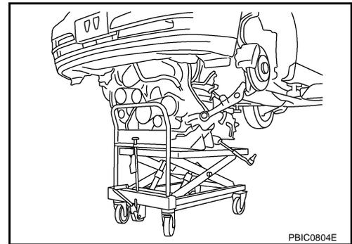
2. Remove rear engine mounting member bolts.
