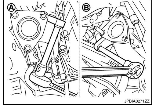
10. Remove exhaust manifold cover (upper) (bank 1 and bank 2).
