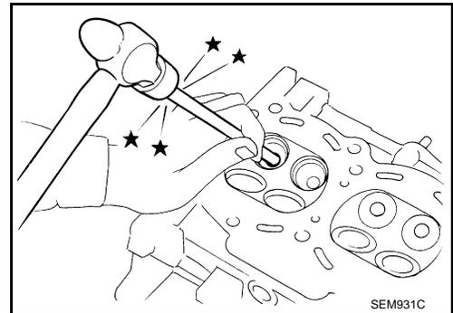
11. Remove spark plug tube, as necessary.
