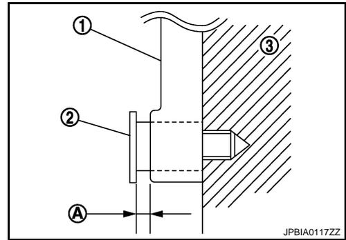
6. Install the timing chain tensioner (primary) with the following procedure:
