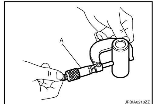
Connecting Rod Bushing Oil Clearance
