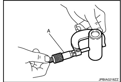
Piston to Piston Pin Oil Clearance
