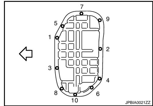
2. Install oil pan drain plug.
