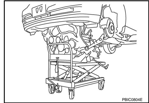
2. Remove rear engine mounting member bolts.
