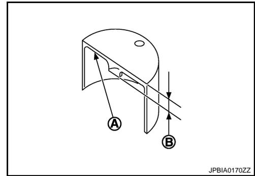
Available thickness of valve lifter: 27 sizes with range 7.88 to 8.40 mm (0.3102 to 0.3307 in) in steps of 0.02 mm (0.0008 in) (when manufactured at factory). Refer to [EM-140, "Camshaft"](#).
