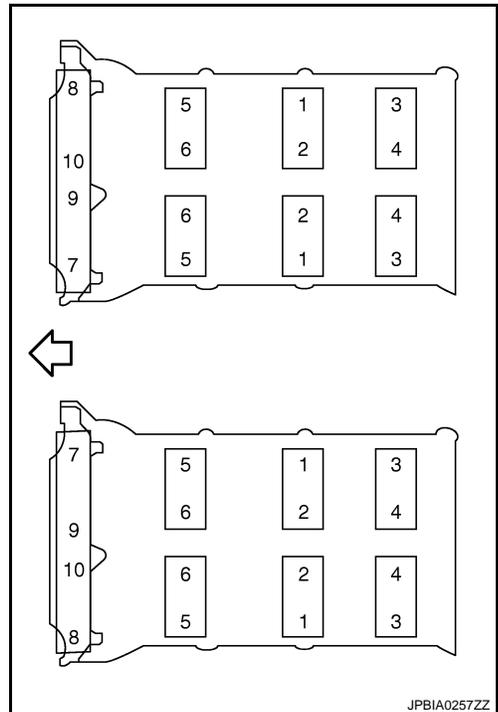
6. Tighten camshaft sensor bracket bolts in numerical order as shown in the figure.
