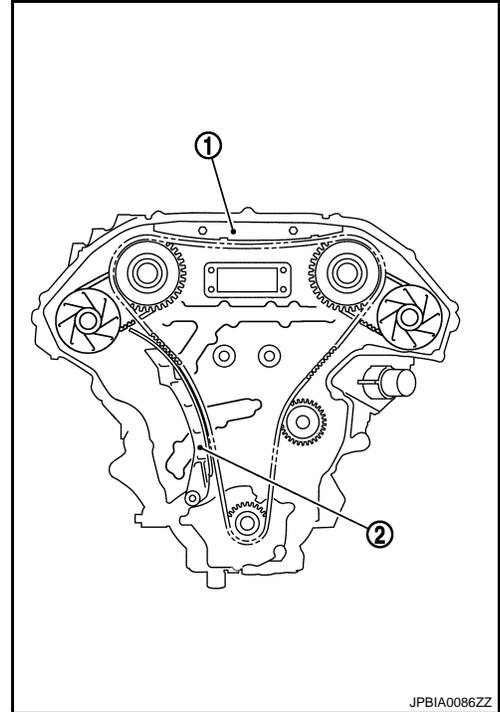
34. Remove timing chain (primary) and crankshaft sprocket.
