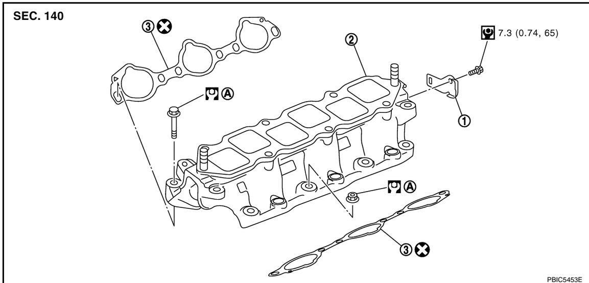
1. Harness bracket                      2. Intake manifold                      3. Gasket
