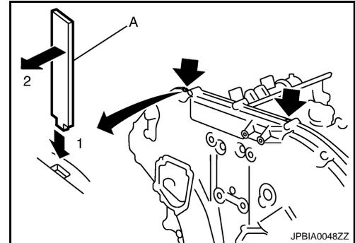
30. Remove front oil seal from front timing chain case using a suitable tool.
