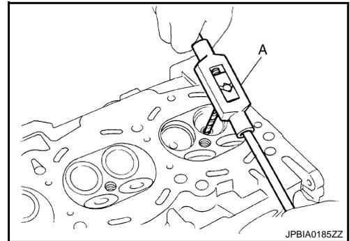
2. If valve seat is removed in step 9 (DISASSEMBLY), install it. Replace with oversize [0.5 mm (0.020 in)] valve seat.
