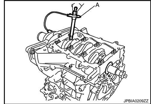
15. Install baffle plate.
