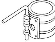
Installing piston assembly into cylinder bore                                                                                                                                                                   |
