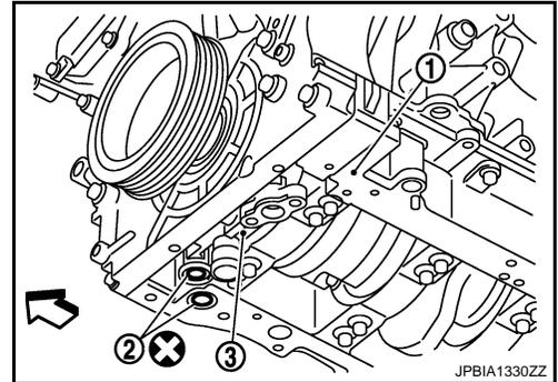
7. Remove axle pipe, as necessary.
