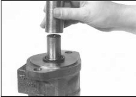
Install dirt & water seal
