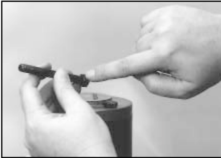
Remove and inspect bolts
