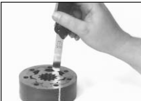
Inspect rotor set
