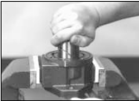
Install coupling shaft
