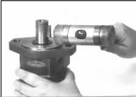
Install shaft hardware
