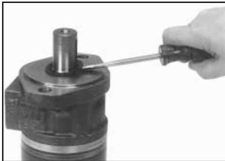
Remove dirt & water seal
