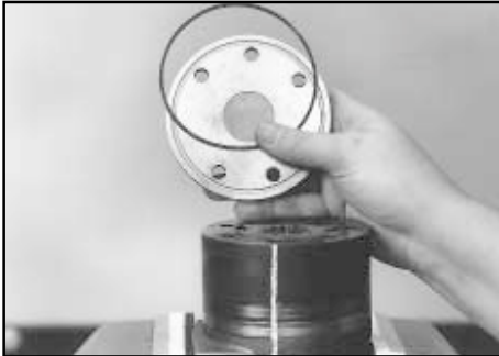
Remove and inspect end cover
