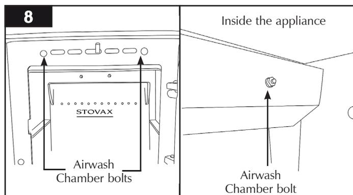
2.3 • Rotate and pull the Airwash chamber through the front of the appliance to remove, Diagram 9
