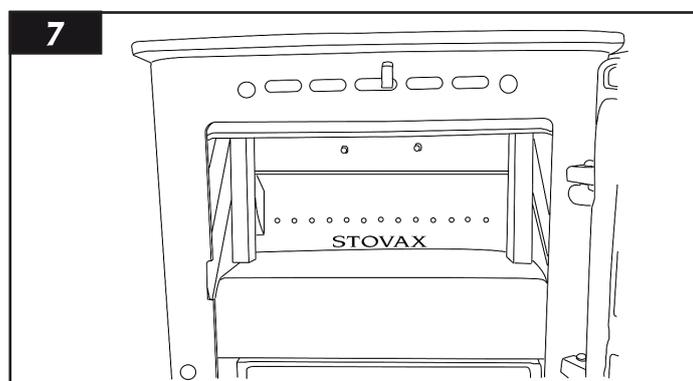
2.2 • Remove the two bolts on the Airwash chamber
