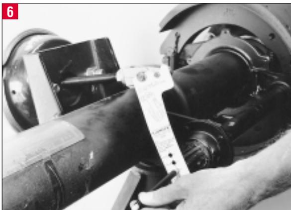
Align the clevis on the threaded push rod until the appropriate centering hole on the template aligns with the center hole on the camshaft. The template is provided with centering holes for 5, 5.5, 6 and 6.5 inch slacks.
