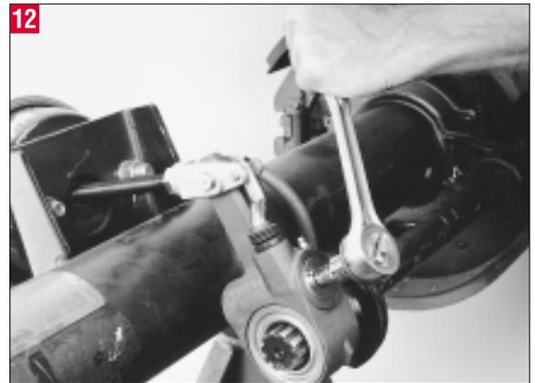
Pre-adjust the brakes by rotating the hex extension clockwise until the brake lining contacts the brake drum. Back the slack adjuster off by rotating the hex counterclockwise 1/2 turn. Backing off a new slack adjuster may require up to 50 ft lbs of torque. A ratcheting sound will be heard when backing the slack off.
