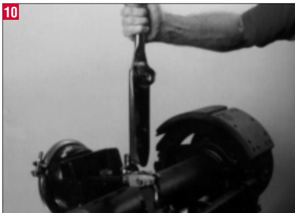
Using a torque wrench, tighten the 1-1/4" collar nut to the clevis using 40 to 50 ft lbs of torque.
