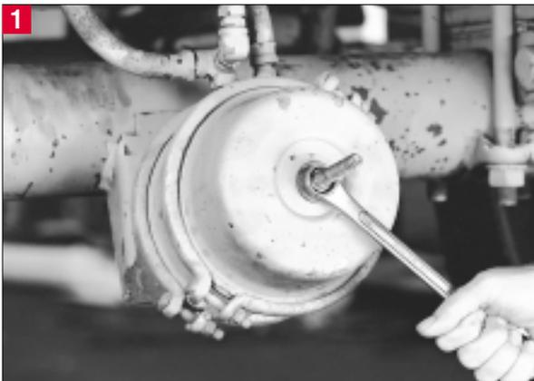
Block the vehicle's wheels. If the axle is equipped with spring brakes, manually cage the brakes following the manufacturer's recommended procedures.
