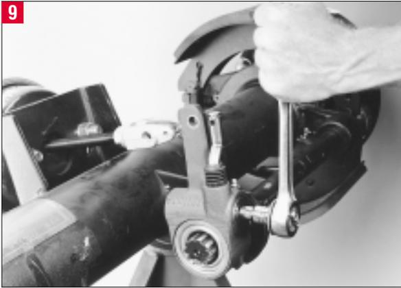
Apply anti-seize compound to the camshaft, install the slack adjuster and adjust the position of the slack using the hex extension. Adjust the slack until the holes in the slack housing align properly with the corresponding holes in the clevis.
