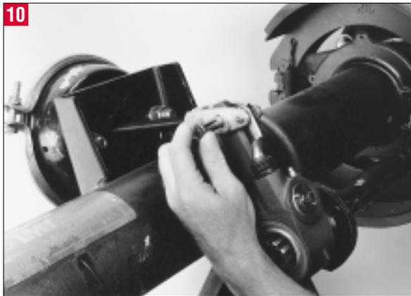
Once the clevis is properly aligned with the slack adjuster, insert both the large and small clevis pins and secure with the cotter pins supplied.
