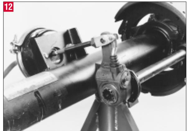
Fully apply the brakes and allow the chamber push rod to travel its maximum stroke. Clearance must exist between the slack adjuster and all adjacent chassis components. Release the brakes.
