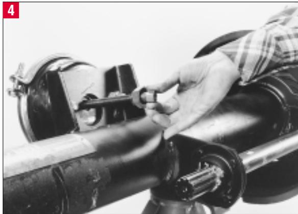
When installing a Gunitite slack adjuster with a collar lock clevis, place the 1-1/4" collar nut on the push rod against the 15/16" jam nut. Next thread the 3/4" hex nut onto the push rod.
