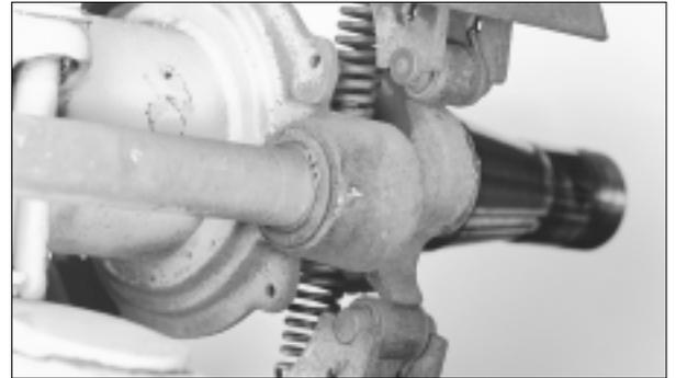
5. After the brake drum has been removed; rotate the hex extension clockwise until the cam turns over. This will allow the brake rollers to be in the release position.
