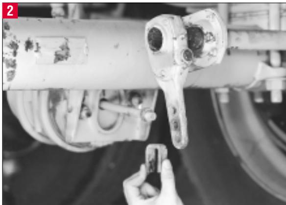
Remove the existing clevis and slack adjuster. Keep the existing mounting hardware. Do not remove the clevis jam nut.
