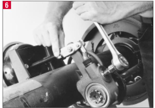
Using the hex extension and a wrench, adjust the slack so that the collar nut aligns with the threaded area of the clevis.
