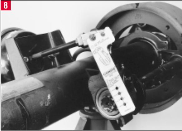
After threading the 1-1/4" collar nut onto the clevis housing, place the template over the large and small clevis pins as shown above.
