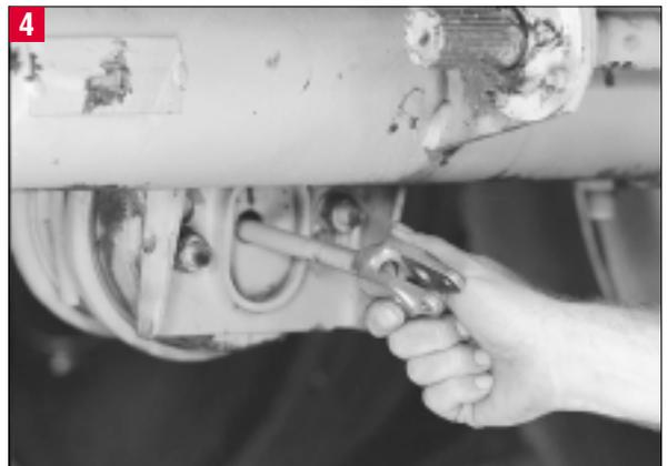
When installing a Gunitite slack adjuster with a threaded clevis, install the new clevis on the push rod in the same location as the clevis which was removed. Do not tighten the jam nut at this time.
