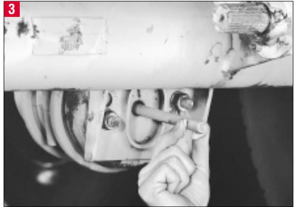
Apply anti-seize to the chamber push rod threads before installing the new clevis.
