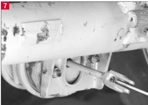
Inspect the clevis installation to make sure that the threaded push rod extends no more than 1/16" past the end of the opening of the clevis in the clevis housing. If the push rod extends more than 1/16" past the clevis housing, the clevis must be removed and the push rod cut to the proper length.
