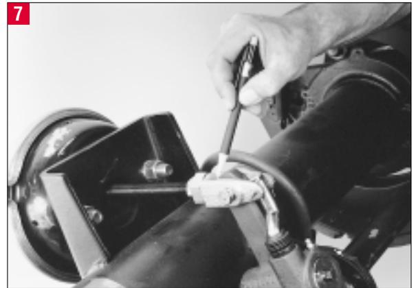
Before attaching the 1-1/4" collar nut to the clevis, check to make sure the threaded push rod is fully engaged in the 3/4" hex nut. If the push rod does not have full engagement, a new push rod must be installed and cut to length. Refer to the section on cutting a new pushrod to length in the service manual.
