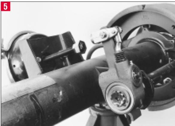
Install the slack onto the camshaft using the original mounting hardware.
