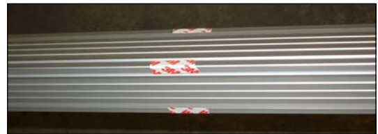
Fig 11.1.D - Apply the adhesive tape you previously cutted to smaller pieces in the MIDDLE of the prism on each side.
