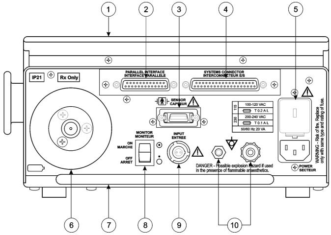
Degree of protection against ingress to solids and water provided by the enclosure.
